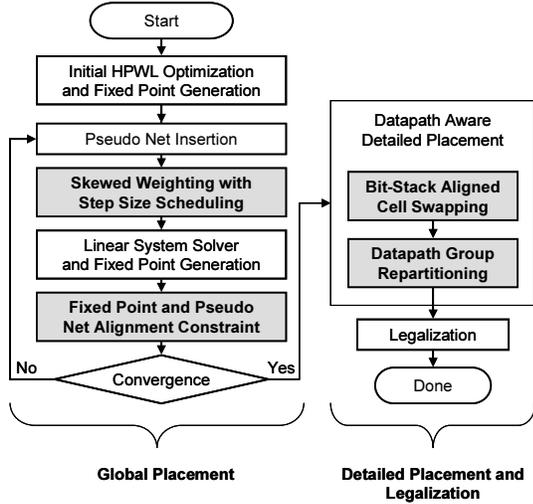
Figure 2: Proposed unified datapath-aware placement flow. The baseline components are shown in transparent boxes and the added datapath-aware components are shaded.
