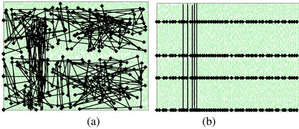
**Figure 7: Forty structured bit-stacks are randomly chosen to show the impact of the proposed placer on structured nets in Benchmark A. (a) is generated by SimPL [16] whereas (b) is generated by the proposed placer. Movable cells are shown lightly shaded while the bit-stack connectivity is shown in black.**
