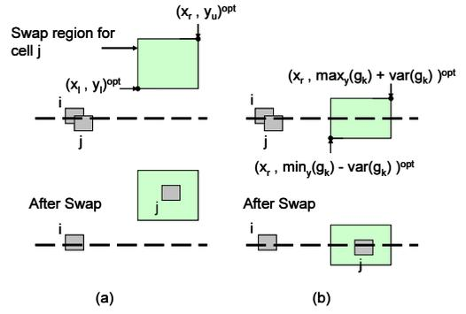
**Figure 5:** Swap region shift for cell  $j$  when the datapath direction is parallel to the  $x$ -axis. The upper  $y$  coordinate location is defined by cell  $i$  plus the variance between cell  $i$  and cell  $j$ .
