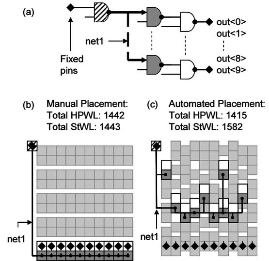
**Figure 1: An example circuit where StWL of the manually placed design is better than that of the automated placement, but HPWL of the automated placement solution is better than that of the manual placement. Net1 has fanout of 10.**
