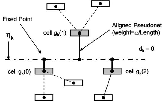
**Figure 4:** Example of a fixed-point alignment constraint for a horizontal bit-stack. Lookahead legalization generates new zero area fixed-points and the locations of these points are modified to be in alignment with  $\eta_k^n$ .
