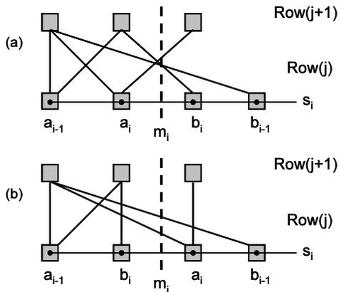
**Figure 6: Group repartitioning example swapping the positions of cell  $a_i$  and  $b_i$  for an improved net cut.**
