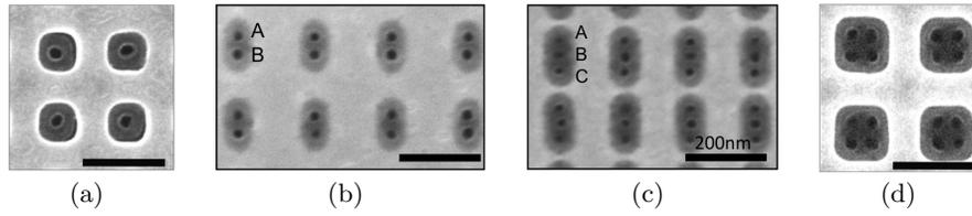
**Figure 2: Regular DSA guiding templates SEM images [10]: (a) single-hole template, (b) two-hole template, (c) three-hole template, (d) four-hole template. [Copyright © SPIE, used with permission]**
