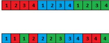
**Figure 4:** Interleaving example; The top row shows the placement before interleaving. The bottom row is the placement after interleaving
