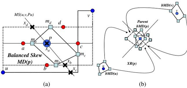
Fig. 6. (a) the balanced skew merging diamond  $bMD(p)$  is constructed with balanced delay points  $m_a, m_d, m_c$ , and  $m_d$ ; (b) parent balanced skew merging diamond  $bMD(p)$  is constructed from two child merging diamonds  $bMD(u)$  and  $bMD(v)$ .
