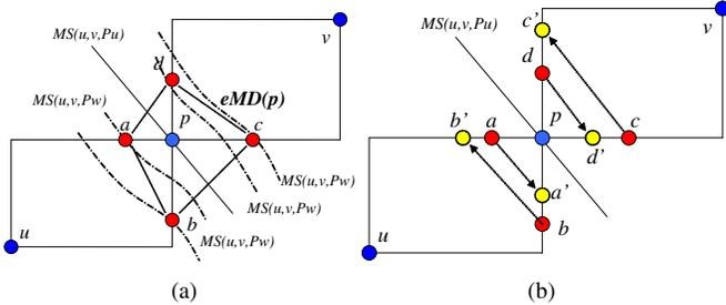
Fig. 4. (a) each equal delay point of  $eMD(p)$  is on  $MS(u,v,P_w)$ ; (b) four points  $a'$ ,  $b'$ ,  $c'$  and  $d'$  are projected from  $a, b, c$  and  $d$  respectively based on the temperature locality to make  $eMD(p)$  smaller.
