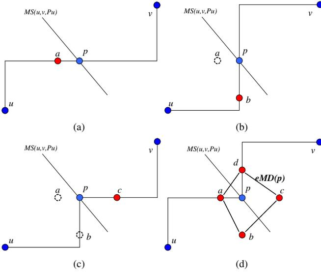
Fig. 3. (a-c) an equal delay point  $a/b/c$  is found along a given path between two children,  $u$  and  $v$ ; (d) an equal delay point  $d$  is found and an equal delay merging diamond  $eMD(p)$  is constructed.
