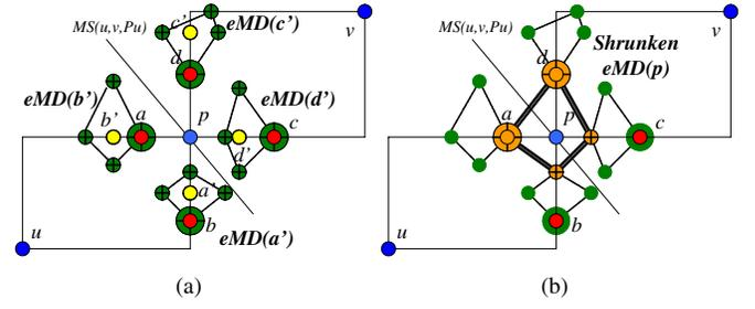
Fig. 5. (a) merging diamonds  $eMD(a')$ ,  $eMD(b')$ ,  $eMD(c')$  and  $eMD(d')$  are constructed around projected points  $a'$ ,  $b'$ ,  $c'$  and  $d'$ ; (b) the shrunken  $eMD(p)$  is constructed with the selected equal delay points.
