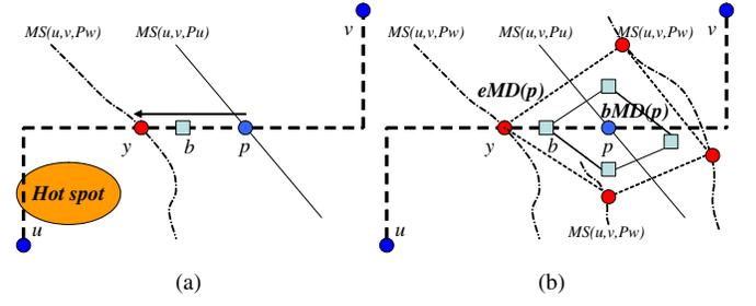
Fig. 1. (a)  $MS(u, v, P_u)$  denotes a merging segment under uniform thermal profile and  $MS(u, v, P_w)$  denotes a merging segment under worst case thermal profile. Equal delay point location moves from point  $p$  to point  $y$  as hot spot appears; (b)  $eMD(p)$  is due to equal delay points on  $MS(u, v, P_w)$  and  $bMD(p)$  is due to balanced skew points (shown as square points).
