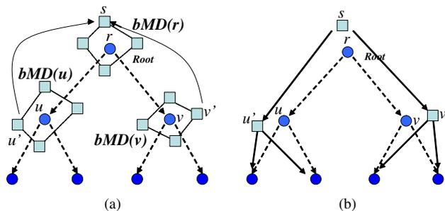
Fig. 2. (a)  $bMD(r)$  is constructed with two child merging diamonds  $bMD(u)$  and  $bMD(v)$  in bottom-up manner. Point  $s$  of  $bMD(r)$  is due to point  $u'$  and  $v'$ ; (b) a point  $s$  with the smallest worst case clock skew from  $bMD(r)$  is selected as a new root and its corresponding tree is traversed in top-down manner.
