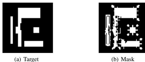
Figure 1. Mask patterns generated from ILT can be extremely complicated with many small features and SRAFs [11].
