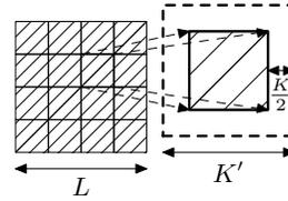
Figure 3. A chip with size  $L \times L$  is divided into many tiles of size  $K' - K$ , where  $K$  is the same as that of sparse simulation and  $K'$  is a tunable parameter. Each tile is zero-padded to of size  $K'$ .
