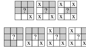
Figure 12. Lithography friendly removable (upper row) and insertable (lower row) pixels, marked by “?”. There are totally 208 cases.
