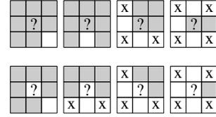
Figure 9. Removable (upper row) and insertable (lower row) pixels (denoted by “?”). There are totally 232 cases.
