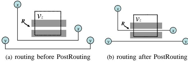
Fig. 17. Example of PostRouting is shown. In (a), a routing capacity  $R$  is not utilized by BoxRouting, as AMR finds less congested path. If  $R$  remains unused after BoxRouting is finished, it may be the reason for suboptimal routing path for a wire  $x$ . Thus,  $x$  can be rerouted by utilizing  $R$ , which shortens a wire  $y$  with the released routing capacity from  $x$  as well, as in (b).
