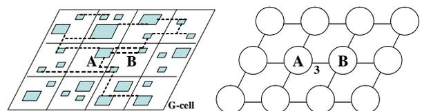
(a) real circuit with G-cells (b) grid graph for routing
