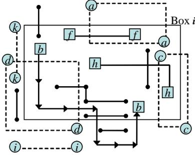
(d) Unrouted wire  $b$  after progressive ILP is routed by adaptive maze routing.
