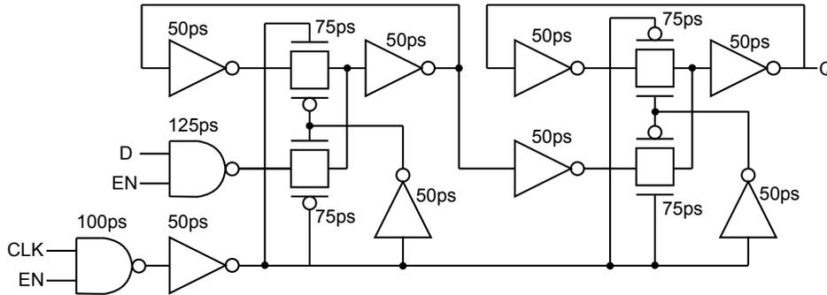
2. (a) Find the setup time, hold time and clock-to-Q delay of the pulse-flip-flop below.
