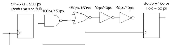
(b) What is the maximum frequency at which the following design can operate?
