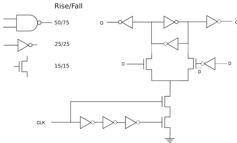
(b) Add one (or more) of the cells shown on the left of the flip-flop in (a) to reduce the setup time to 0 (or less), without changing the circuitry already in place.
