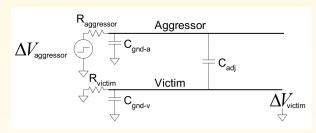
$$\Delta V_{victim} = \frac{C_{adj}}{C_{gnd-v} + C_{adj}} \frac{1}{1+k} \Delta V_{aggressor}$$
