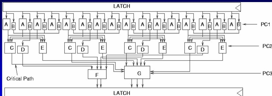
Use structure of circuit and delay to determine the **longest structural path** in block (could be a **false path**)
