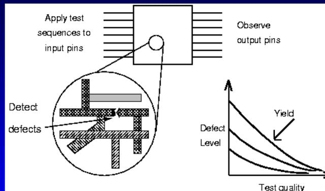
A **test** for a defect will produce an output response which is different from the output when there is no defect
