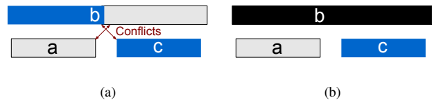
Fig. 2: (a) In DPL, even stitch insertion can not avoid native conflict. (b) The native conflicts can be resolved by TPL.
