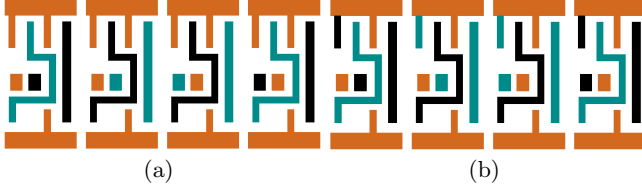
Figure 7: AND2X1 pre-coloring solutions with (a) 0 stitch; (b) 1 stitch.
