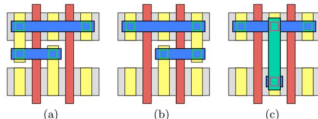
**Figure 5: An example of P/N terminals connection for a net. (a), (b), and (c) are the three possible routes for the net with two P-terminals and one N-terminal.**
