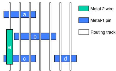
Figure 2: An example of pin access value calculation.
