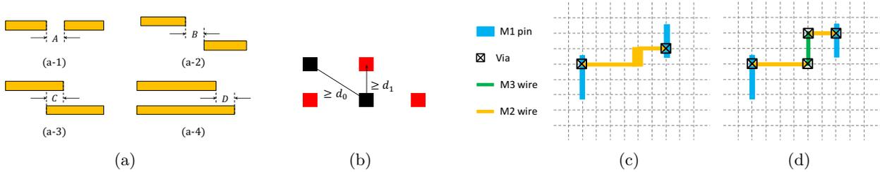
Figure 3. (a) Line-end design rules for SADP, (b) LELE coloring rules for via patterns, (c) 2D routing patterns with restrictive design rules, (d) 1D routing patterns with extra vias.<sup>4,11,20</sup>
