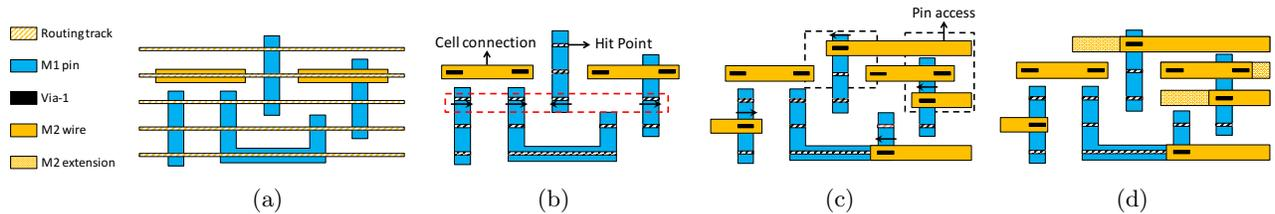
Figure 5. Standard pin access optimization, (a) standard cell I/O pins and M2 routing tracks, (b) hit points and M2 within-cell connections, (c) a hit point combination with M2 pin access, (d) SADP-friendly pin access with M2 extensions.<sup>4</sup>
