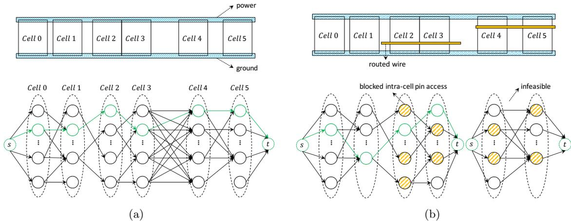
Figure 8. Global pin access planning with single row pin access graphs, (a) initial pin access graph, (b) updated pin access graph with graph simplification and routed M2 wires.<sup>20</sup>
