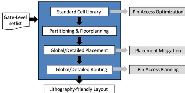
Figure 4. Overall physical design flow for pin accessibility optimization in advanced lithography.
