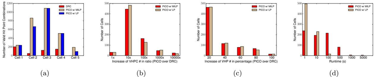
Figure 10. Standard cell pin accessibility improvement from PICO, (a) increase in number of VHPCs for different cells, (b) increase of VHPC # in ratio across the entire library, (c) increase of VHP # in percentage across the entire library.
