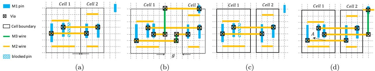
Figure 2. Placement and routing level impacts on standard cell pin access, (a) two cells placed next to each other, (b) two cells placed with a gap of three placement pitches, (c) pin access failure during detailed routing, (d) pin access success during detailed routing.<sup>20</sup>
