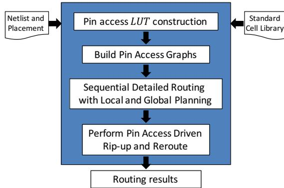
Figure 9. Overall detailed routing flow.
