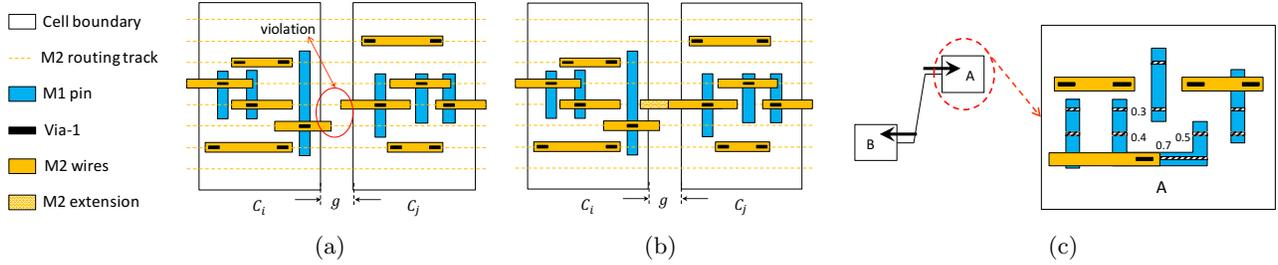
Figure 7. (a) Inter-cell pin access interference with a violation, (b) fix the violation by line-end extension, (c) local pin access planning with dynamic hit point scoring.<sup>20</sup>
