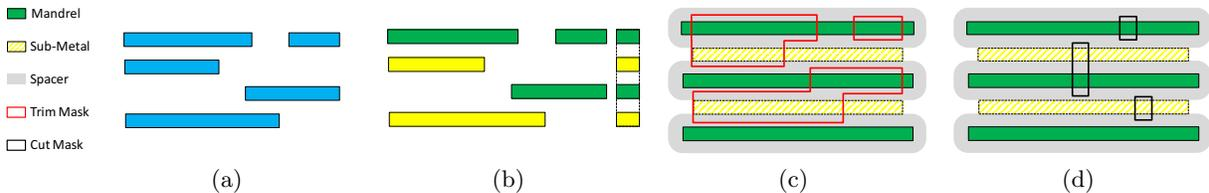
Figure 1. Track-based coloring for unidirectional layout patterns with SADP, (a) unidirectional target patterns, (b) track-based coloring, (c) SADP with trim masks, (d) SADP with cut masks.<sup>20</sup>
