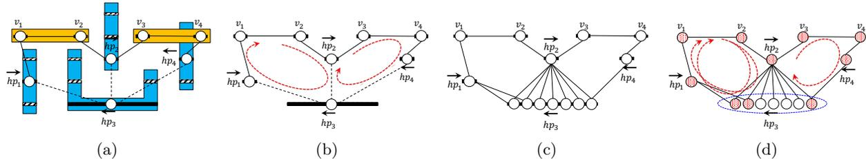
Figure 6. LELE-aware via-1 assignment, (a) standard cell I/O pins and via-1's for within-cell connections, (b) conflict graph for hit points and via-1's, (c) conflict graph with grid-based segmentation for long hit points, (d) odd cycles in the conflict graph.<sup>4</sup>
