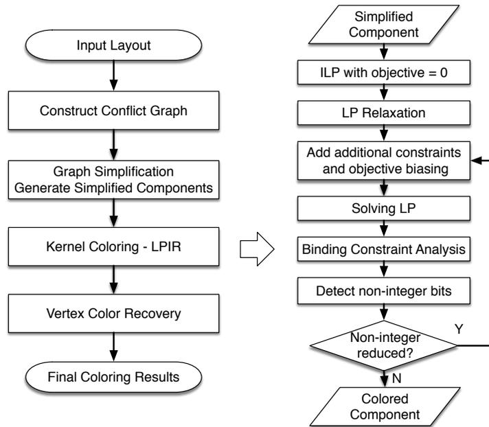
Figure 3. Overall flow for our coloring framework.
