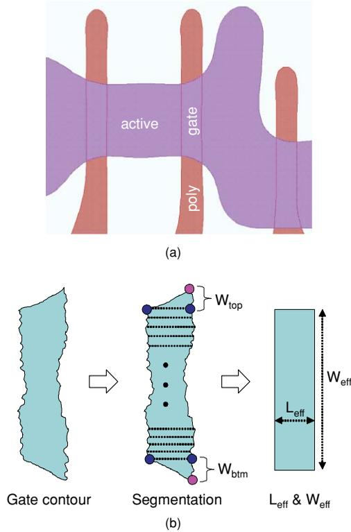
**Fig. 5** Gate segmentation approach for an effective gate length: (a) poly and active printed images induce nonrectangular gates and (b) calculation of an effective gate length from a nonrectangular gate with LER.
