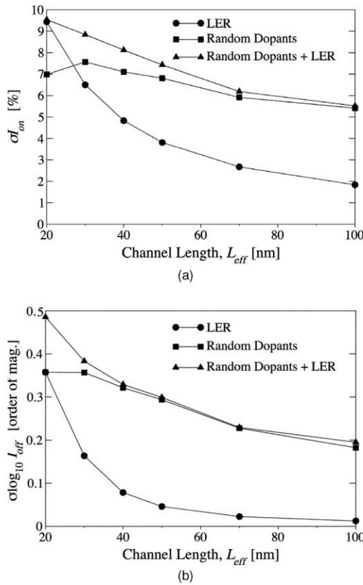
**Fig. 1** Impact of line edge roughness:<sup>13</sup> (a) dependence of  $I_{on}$  on the channel length, and (b) dependence of  $I_{off}$  on the channel length. The RMS amplitude of LER is 2 nm for all cases.
