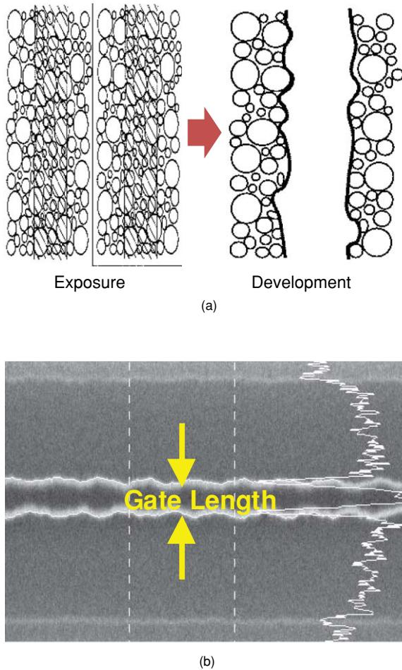
**Fig. 3** Random LER lithography variation: (a) mechanism of LER generation<sup>21</sup> and (b) wafer scanning electron microscopy (SEM) image of gate LER (Ref. 16).
