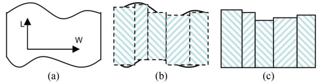
Fig. 2. Nonrectangular gate and slicing for electrical analysis [33]. (a) Nonrectangular gate after printing. (b) Gate is sliced into small pieces along the channel. (c) Each slice will be modeled by its equivalent gate length. They will be combined to get the equivalent gate length for the original gate.
