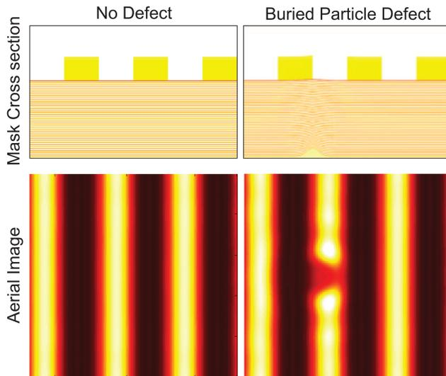
Fig. 22. EUV buried defect on a mask and the simulated aerial images [126].
