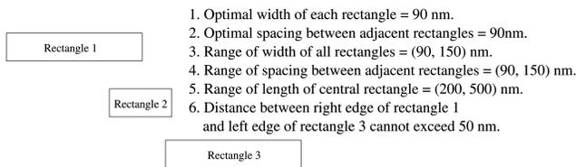
Fig. 4. Example of range pattern staircase [39].
