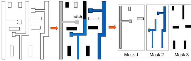
Fig. 14. Layout decomposition for triple patterning lithography (TPL).
