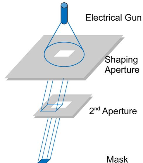
Fig. 23. Variable shaped beam (VSB) is a conventional EBL technique.
