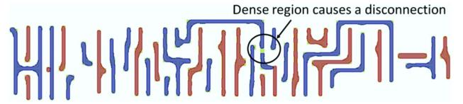
Fig. 10. Unbalanced decomposition may have a pattering problem [67].
