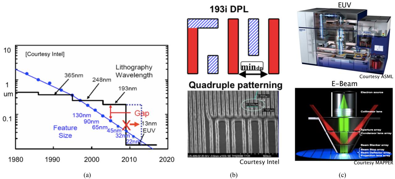
Fig. 1. (a). The lithography roadmap and EUVL delay. (b) The 193nm extension with double patterning or even quadruple patterning. (c) Other next-generation nanolithography technologies such as EUVL and EBL.
