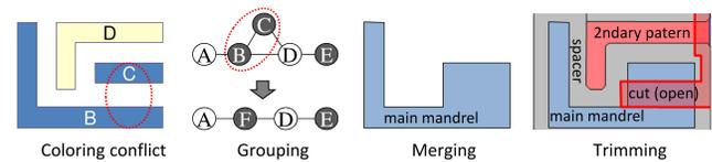
Fig. 13. Grouping and merging coloring for spacer-based multiple patterning [74].
