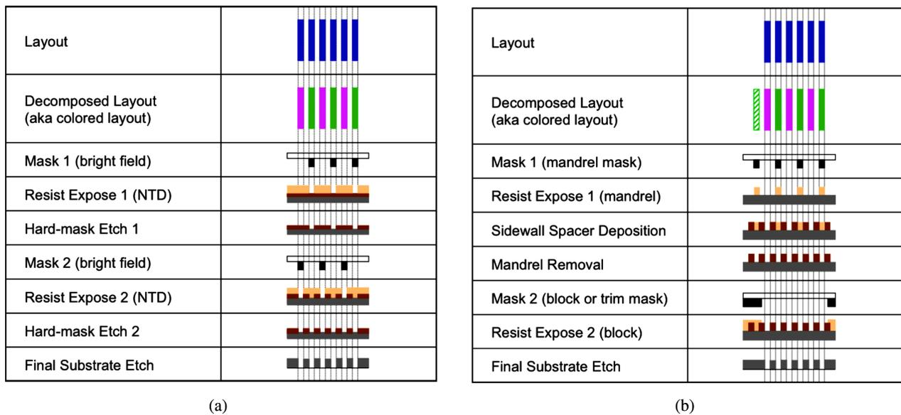
Fig. 7. Manufacturing processes of the two main double patterning lithography technologies. (a) LELE. (b) SADP. (Courtesy of IBM.)
