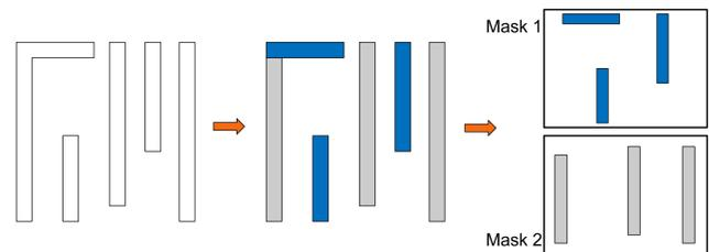
Fig. 8. Example of LELE layout decomposition.
