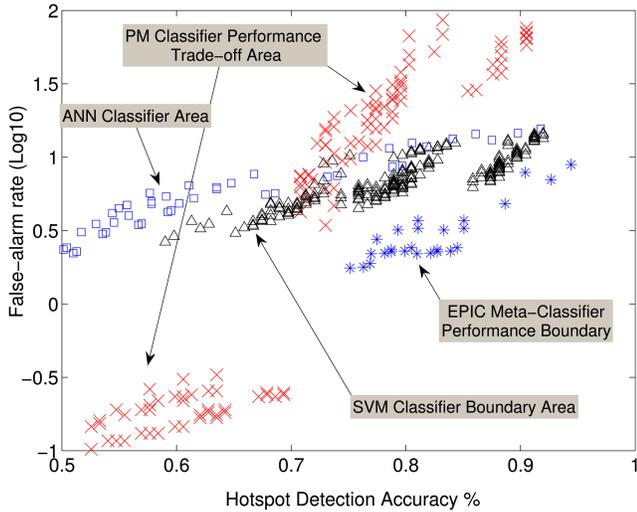
Fig. 6. Tradeoff between hotspot accuracy and false-alarm using various pattern matching and machine learning methods [36].
