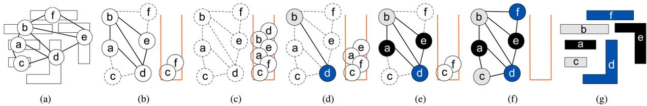
Fig. 15. Iterative vertex removal [81]. (a) Conflict graph. (b) and (c) Iteratively remove and push in vertices with degree no more than two. (d)–(f) After color assignment for the remanent vertices, iteratively pop up and recover vertices, and assign any legal color. (g) Layout decomposition can be finished after the iterative vertex recover.
