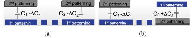
Fig. 11. (a) Layout decomposition without considering overlay compensation. (b) Layout decomposition considering overlay compensation [67].
