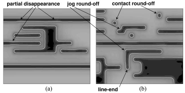
Fig. 3. (a) and (b). Two examples of lithography hotspot patterns [36].
