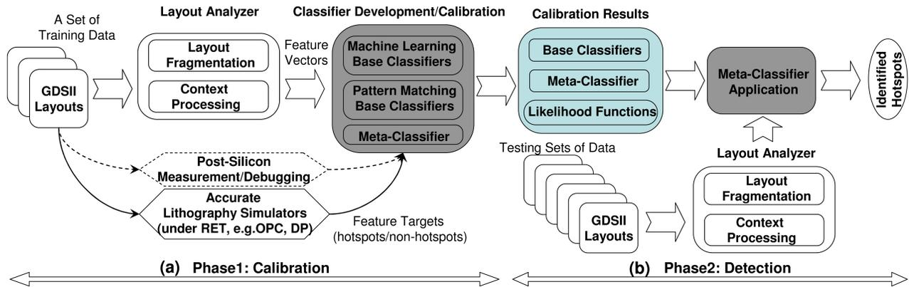
Fig. 5. Overall CAD flow proposed in [36] for hotspot detection based on metadetection formulation.
