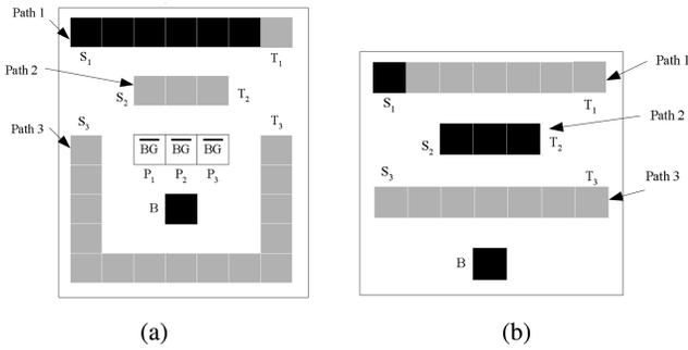
Fig. 18. DPL-aware routing with lazy routing [104]. (a) Coloring together with routing may cause detour. (b) Lazy coloring reduces wirelength.
