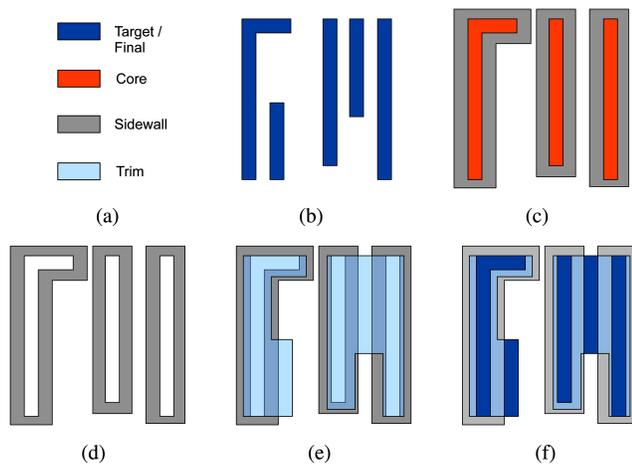
Fig. 12. SADP process of generating some sample 2-D layout. (a) Some labels. (b) Target features. (c) Core patterns and spacers generation. (d) Spacers after core patterns removal. (e) Trim mask. (f) Final patterns.
