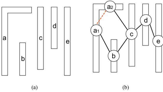
Fig. 9. (a) Given input layout. (b) Constructed conflict graph, where one stitch edge is introduced.
