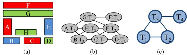
Fig. 20. TPL-aware routing with token graph to represent relative coloring relationship and the graph size. (a) TPL coloring. (b) Conflict graph and token assignment. (c) Token graph [106].
