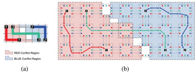
Fig. 19. Triple patterning-aware routing with expanded graph [105]. (a) Routes on the original routing grid. (b) Routes on the expanded routing graph.
