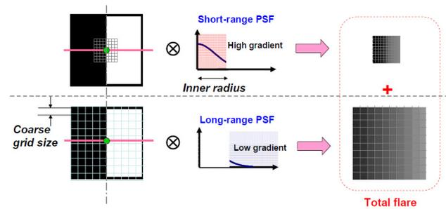
Fig. 21. Total (short and long range) flare kernels in EUV lithography [111].
