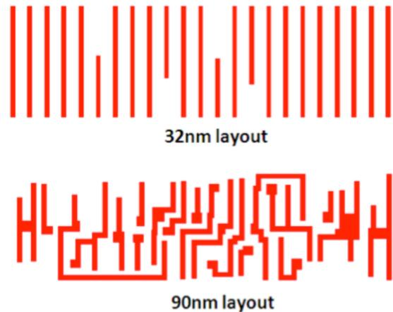
Fig. 17. Poly lines of sample 32-nm and 90-nm layouts (courtesy ARM).
