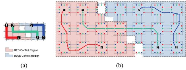
Fig. 19. Triple patterning-aware routing with expanded graph [105]. (a) Routes on the original routing grid. (b) Routes on the expanded routing graph.
