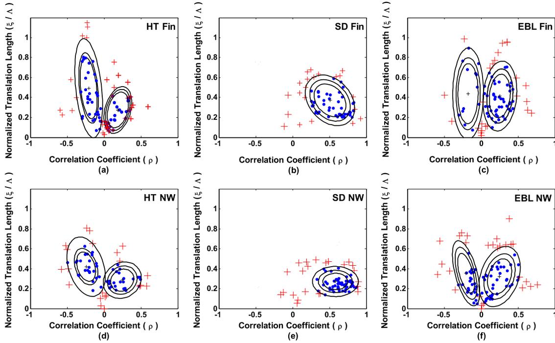
Fig. 5. Normalized translation length ( $\xi/\Lambda$ ) versus correlation coefficient  $\rho$  extracted from experimental results of Fin/nanowire under different patterning techniques. (a) and (d) HT. (b) and (e) SD. (c) and (f) EBL. Fiducial confidence ellipses are drawn in the picture with confidence level of 0.3, 0.5, and 0.7.
