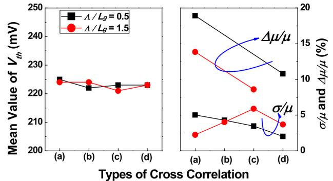
Fig. 13. Four types of cross-correlation share similar mean  $V_{th}$  (left);  $\sigma/\mu$  is smaller than 10% in four cases while  $\Delta\mu/\mu$  is up to 19% (right).
