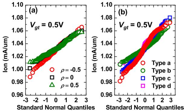
Fig. 14. Q-Q tests of  $I_{on}$ . (a) Conventional simulation. (b) After consideration of cross-correlation.
