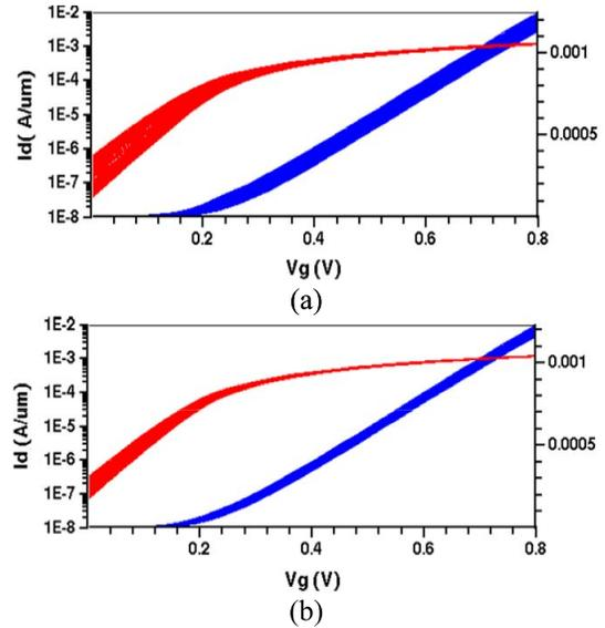
Fig. 8. Transfer characteristics of DG devices with different cross-correlation properties (a)  $\rho = -0.5$  and (b)  $\rho = 0.5$ .
