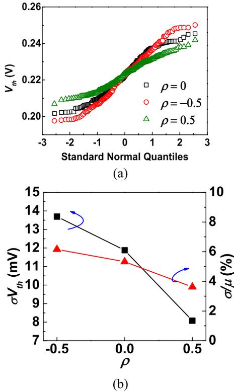
Fig. 9.  $V_{th}$  distribution without considering cross-correlation. (a) The Q-Q test shows that conventional  $V_{th}$  distributions fit well with Gaussian distribution. (b) Normalized deviation of  $V_{th}$  is smaller than 6%.
