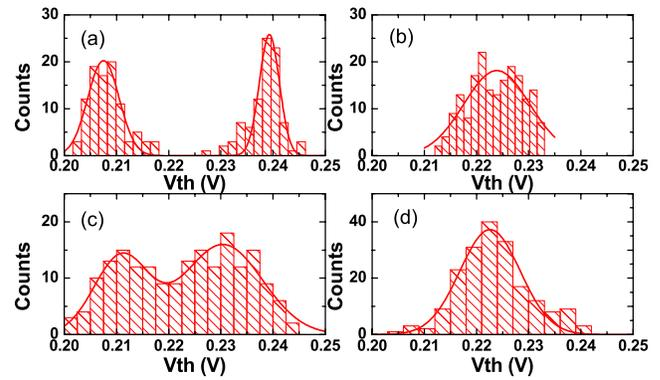
Fig. 11. Distributions of threshold voltage under four types of cross-correlation with  $\Lambda/L_g = 1.5$ .
