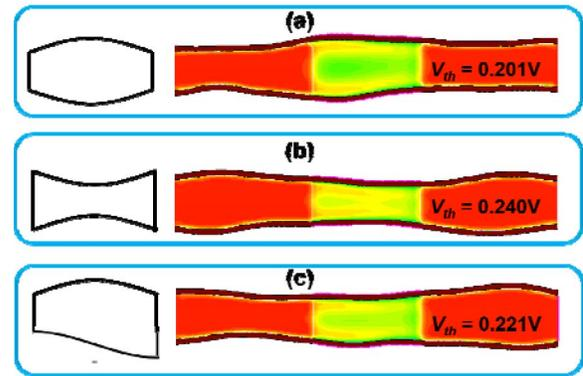
Fig. 12. Explanation for the impacts of cross-correlation condition ( $\Lambda = 10$  nm,  $\rho = -0.5$ ). (a)  $\zeta = 0$ , (b)  $\zeta = 0$ , and (c)  $\zeta = 0.5$   $\Lambda$ .
