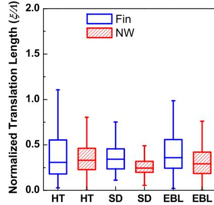
Fig. 4. Box chart of normalized translation length ( $\xi/\Lambda_{\text{eff}}$ ) of Fin/NW LER by different fabrication processes.
