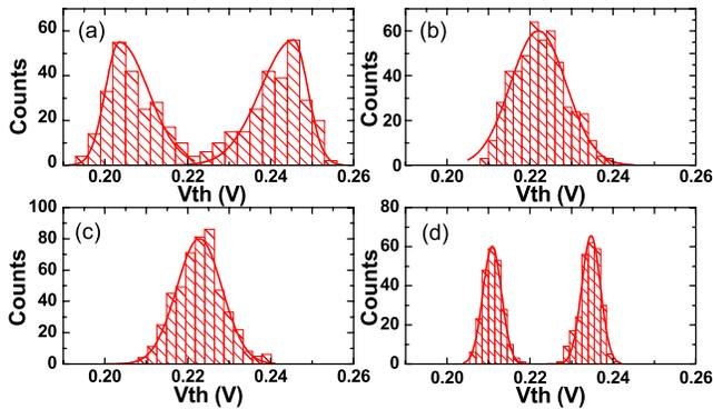
Fig. 10. Distributions of threshold voltage under four types of cross-correlation with  $\Lambda/L_g = 0.5$ .
