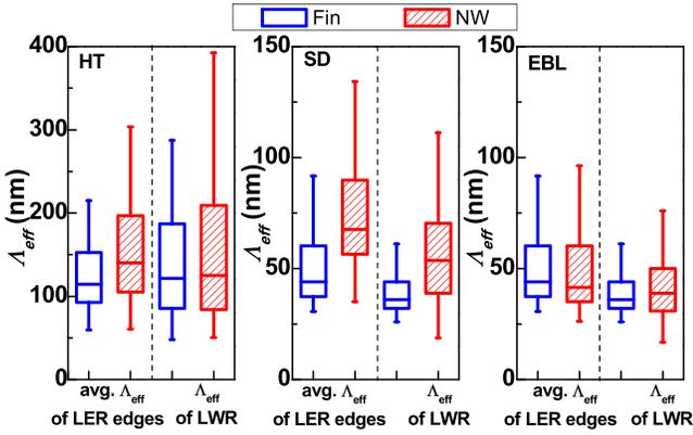
Fig. 2. Box chart of average LER  $\Lambda_{\text{eff}}$  and LWR  $\Lambda_{\text{eff}}$  of Fin and NW fabricated by three different processes.
