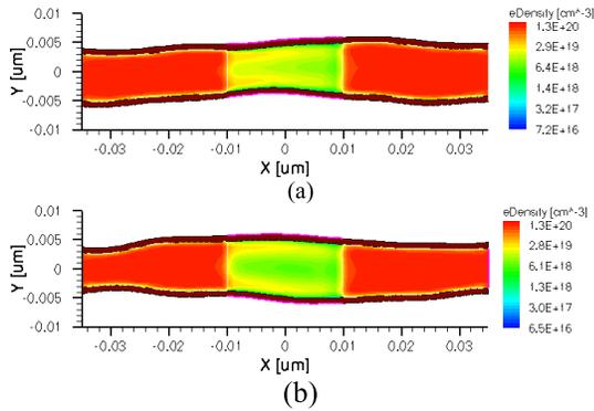
Fig. 7. Electron density distributions of DG devices with  $\Lambda = 10$  nm,  $\xi = 0$ , and (a)  $\rho = 0.5$  and (b)  $\rho = -0.5$ .
