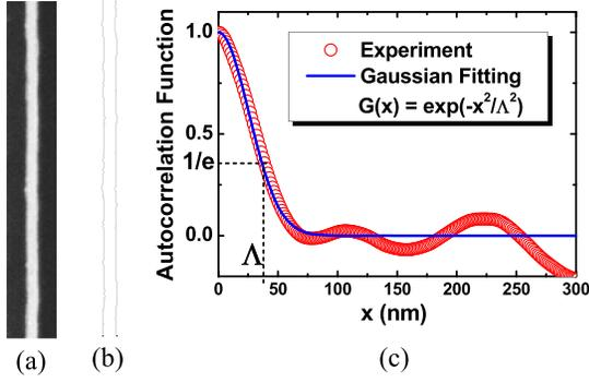
Fig. 1. (a) Top-view SEM image of 40-nm nanowire channel. (b) Edges detected from the SEM image. (c) Auto-correlation function with Gaussian fitting.
