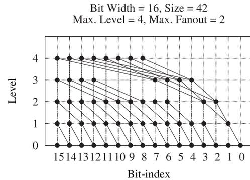
Fig. 15. Size of a 16 bit prefix graph with level 4 and fanout 2 generated by our approach is less than that of Kogge Stone by 7.
