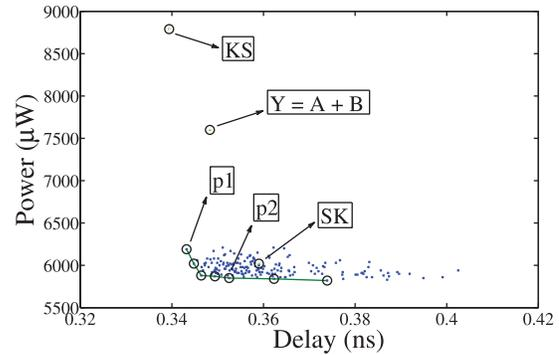
Fig. 18. Delay versus power plot for 64 bit adder.
