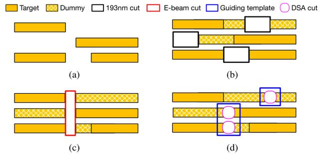
**Fig. 12** Post-routing decomposition with line-end extensions, (a) target patterns, (b) 193 nm cut [16], [56], (c) E-beam cut [7], [10], (d) guiding template with DSA cut [61].
