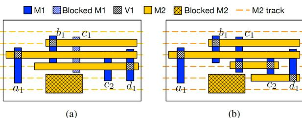
Fig. 7 Pin access interference on M2, (a) pin access failure, (b) pin access success [68].
