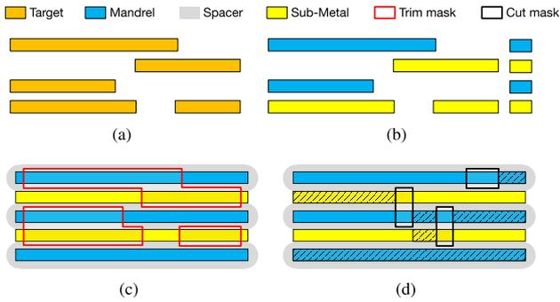
**Fig. 2** (a) Target patterns, (b) track-based coloring, (c) SADP with trim masks, (d) SADP with cut masks [62].
