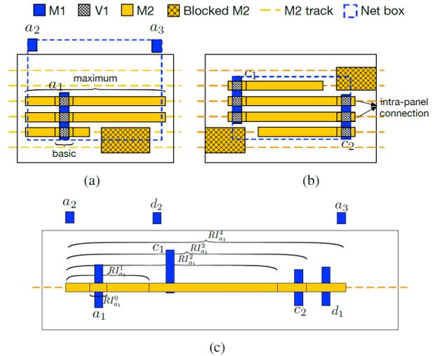
**Fig. 9** Routing interval generation, (a) a pin close to M2 blockages, (b) two pins sharing the same net, (c) handling pin-to-pin interference.
