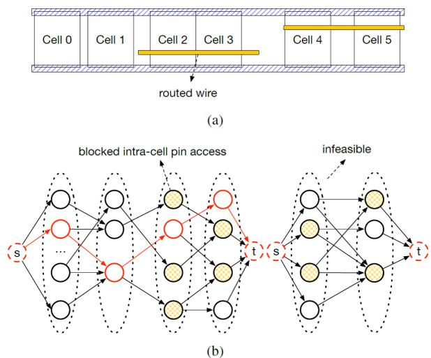
Fig. 8 Single row pin access graph (PAG), (a) cell placement, (b) simplified PAG with routed wires [68], [69].
