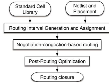
**Fig. 4** Unidirectional routing flow.
