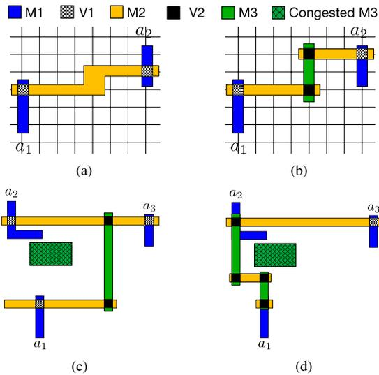
**Fig. 10** (a) Two-dimensional routing, (b) unidirectional routing, (c) more wirelength with routing interval assignment, (d) more vias without routing interval assignment.
