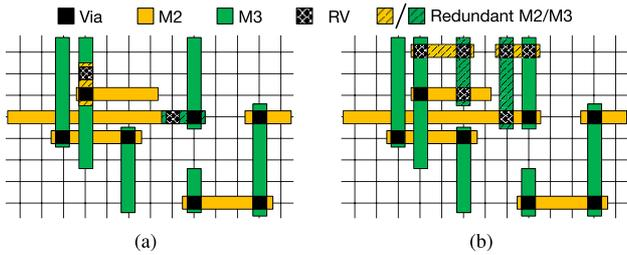
**Fig. 11** (a) Redundant via insertion with wire bending, (b) redundant local loop insertion for unidirectional routing [67].
