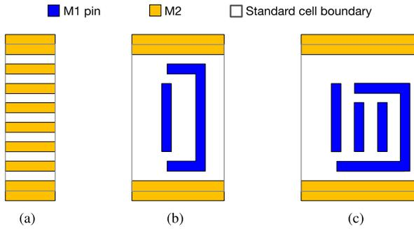
**Fig. 5** Standard cell architecture, (a) 7.5 M2 track architecture, (b) “Inverter” layout on M1 and M2, (c) “AND-OR-Inverter” layout on M1 and M2 [33].
