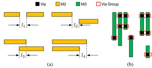
**Fig. 3** (a) Metal line-end design rules [40], [64], (b) self-aligned via groups [3], [53].
