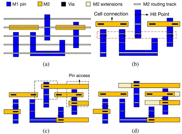
**Fig. 6** (a) M1 I/O pins and M2 routing tracks, (b) hit points and M2 usage for within-cell connections, (c) a hit point combination with M2 pin access patterns, (d) M2 pin access patterns with line-end extensions [64].
