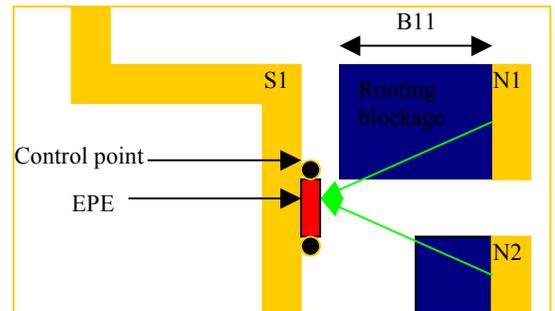
Figure 4: Routing blockage generation for ripup and reroute.
