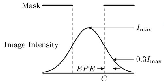
**Figure 2: EPE estimation based on image intensity.**
