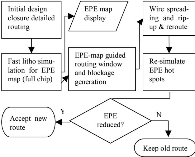
Figure 3: EPE based detailed routing flow (RADAR).
