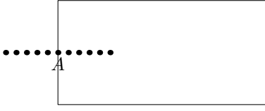
Figure 3. EPE computation requires many intensity simulations. The box is the target shape. To find the printed contour near the tag point A , we may need to simulate on many points.
