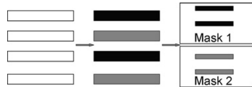
Fig. 1. One single design is decomposed into two masks and the pitch size is increased effectively in DPL.
