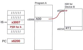
Saved.USP = R6. R6 = Saved.SSP. Push PSR and PC onto stack, then transfer to Device B service routine (at x6200)...
