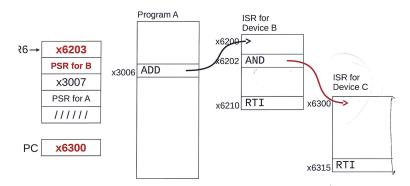
Push PSR and PC onto stack, then transfer to Device C service routine (at x6300).
