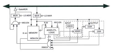
Because of interrupt enable bits, status registers (KBSR/DSR) must be written, as well as read.
