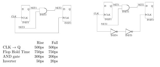
2. (a) Identify if there are any hold time problems from the source flops (G1, G2, G3 and G4) to G11 in the circuit below. If there are any, indicate by how much the hold time is violated and suggest a fix which minimizes the impact on the delay of the circuit. Use the delays from the table below.
