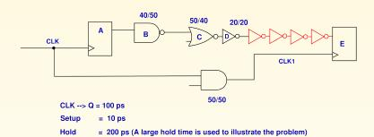
**Insert 4 inverters after D**, with each adding a 20 ps (or can insert one AND gate)
