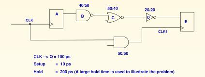
Shortest path delay from A  $\rightarrow$  E = 100 + 40 + 40 + 20 = 200 ps Delay between CLK1 and CLK = 50 ps Adjusted hold time = 200 + 50 = 250 ps Hold Slack = (Path Delay) - (Adjusted Hold Time) = 200 - 250 = -50 ps  $\implies$  FAIL (Hold slack should be  $\geq$  0)
