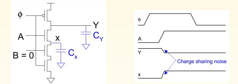
$$V_x = V_y = \frac{C_y}{C_x + C_y} V_{DD}$$
