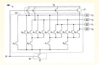
Ref: U. S. Patent 6066965, Method and apparatus for a N-nary Logic Circuit Using 1 of 4 Signals
