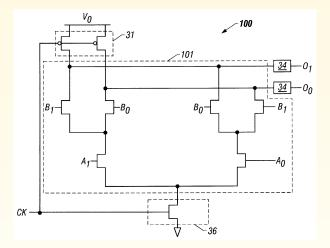
Ref: U. S. Patent 6066965, Method and apparatus for a N-nary Logic Circuit Using 1 of 4 Signals
