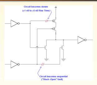
Test for the stuck-open fault at gate of n-channel gate Pattern 11 (followed by)
