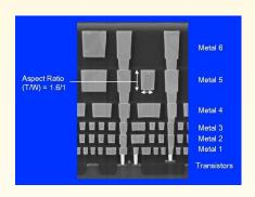
Breaks in Copper interconnect result in resistive opens because the barrier materials preventing interaction of Cu and  $SiO_2$  will still be conductive
