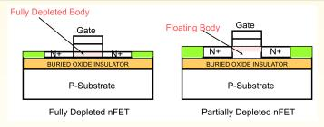
Difficult to manufacture FD devices due to thin Si layer requirement
