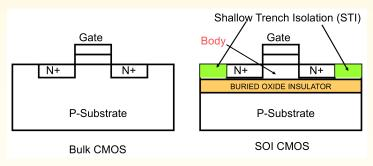
Most of the process tooling is the same for Bulk and SOI SOI devices have 5 terminals – Gate, Drain, Source, Substrate, Body
