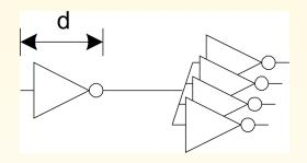
Logical Effort: g=1Electrical Effort: h=4Parasitic Delay: p=1Stage Delay: d=5 The FO4 delay is about: 200 ps in a  $0.6\mu m$  process 60 ps in a 180 nm process f/3 ns in a f  $\mu m$  process (f/3 ps in a f nm process)
