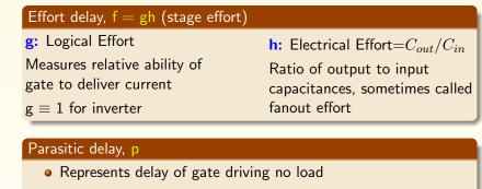
• Set by internal parasitic capacitance
