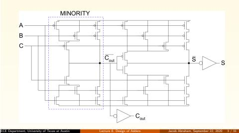
$\bullet\,$  Critical path is usually C to  $C_{out}$  in ripple adder
