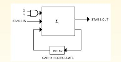
Area for structure increases linearly with number of bits, n
